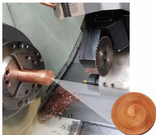
Turn Cut Milling: copper ETP V_c = 300 \text{ m/min} F_z = 0,08 \text{ mm}
