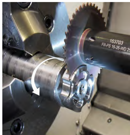
Cutting of VA structured components V_c = 160 \text{ m/min} F_z = 0,1 \text{ mm}
