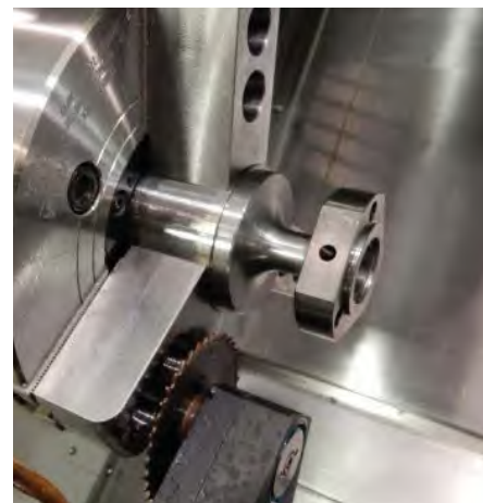
Turn Cut Milling: aluminium V_c = 800 \text{ m/min} \text{feed} = 7 \text{ m / min}
